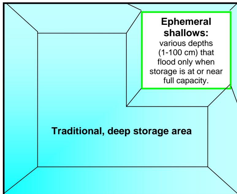
**Figure 5.2** Basic conceptual design to enhance a typical storage dam for Brolgas, other threatened waterbirds and biodiversity generally.
